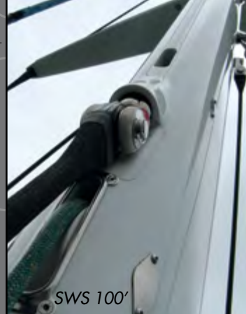
Photo : Marstrom Internal halyard lock on a Gunboat 60'
