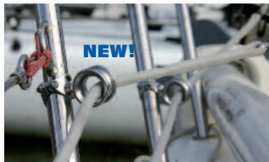
With the different Facnor fairleads, the lines run clearly on the deck Above : articulated fairlead (left handside) et twin fairlead (right handside)
