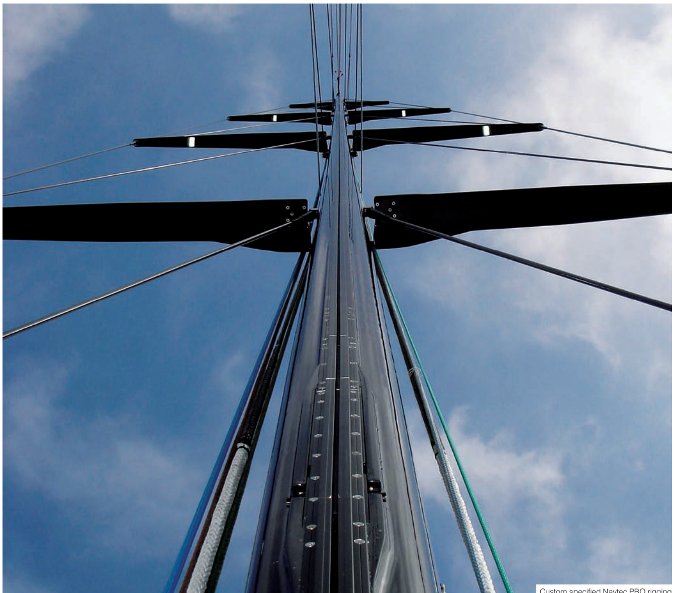
Custom specified Navtec PBO rigging
