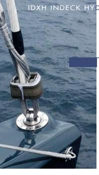
The IDXH hydraulic furler performs similar functions to the FXH model, but it is fitted under the deck or in the bowsprit what makes it invisible and elegantly integrated.
